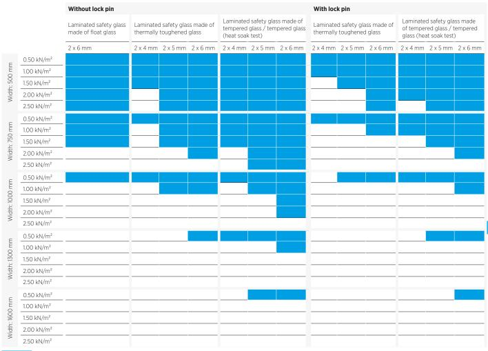
complies with DIN 18008 does not comply with DIN 18008
